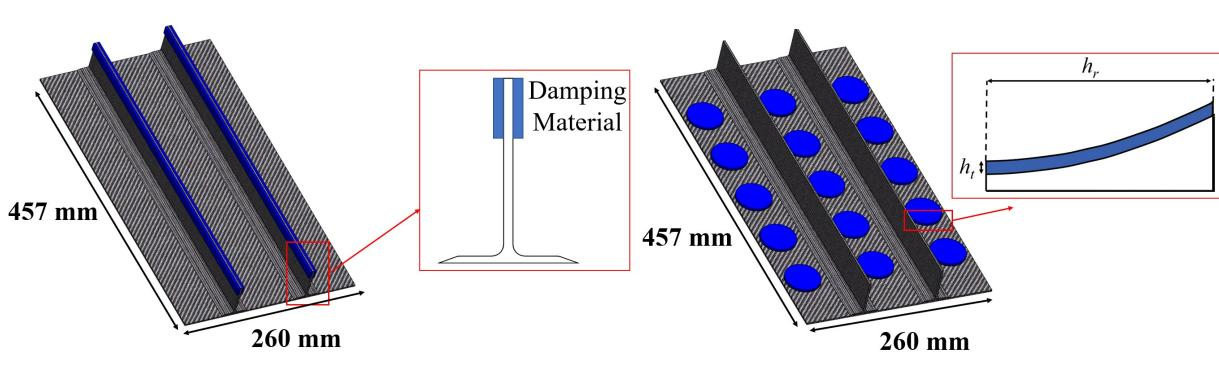
The surface averaged velocity allows the damping effect of the ABHs to be visualized. Above 1500 Hz, distinct peaks can no longer be seen in the ABH design, and the mobility can be ~15 dB lower at certain frequencies.
