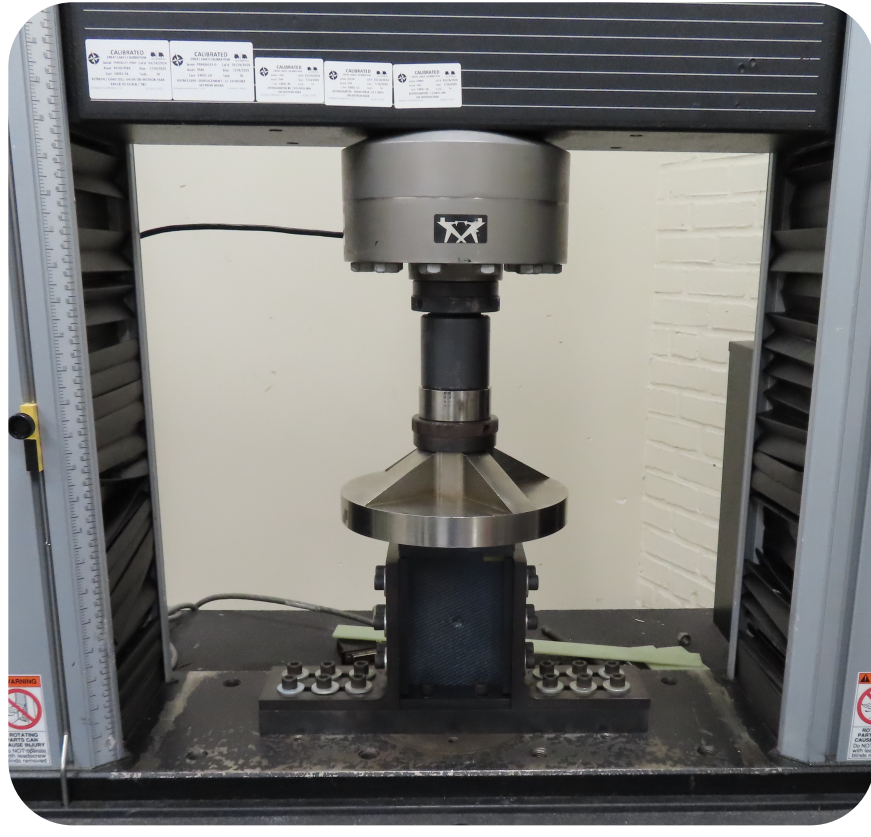
Mechanical Testing: Compression After Impact (CAI) using Instron 5584 Load Frame
