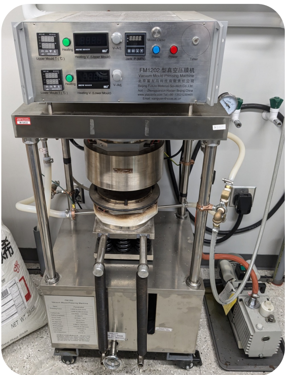
Mould Press: Using 4 MPa and 300 ° C to repair the impacted area
